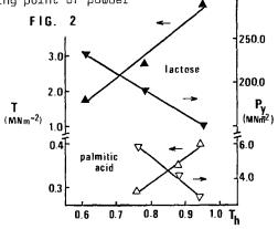
In Fig.1 it can be seen how the slope of each plot increases with temperature indicating a fall in yield pressure of the material; and in Fig.2 how this fall is matched by a corresponding increase in tablet tensile strength. The results show that the temperature of compression has a marked effect on the ultimate mechanical strength of the tablet. This is due to increased interparticular plastic deformation occurring as the yield pressure of the powder particles is reduced.
